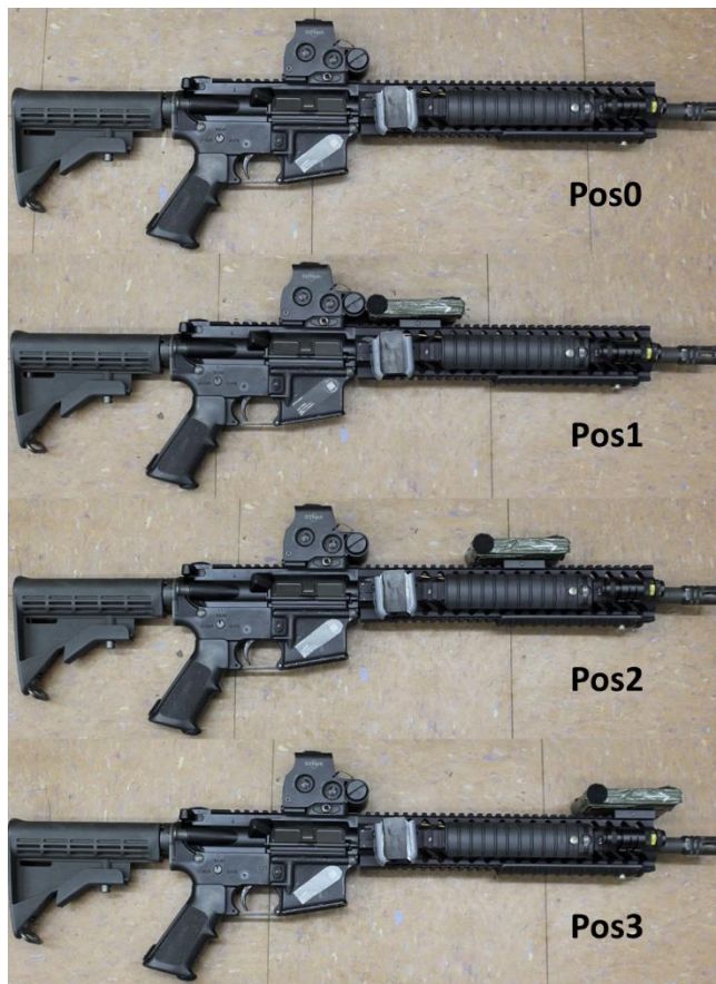
Figure 1 caption. M4 baseline (Pos0), and with mass installed in three positions (Pos1-Pos3, highlighted)
