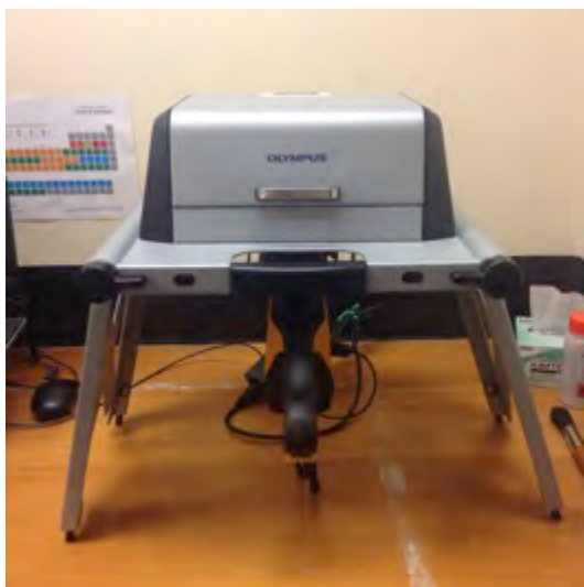
Figure 7. 18 Olympus DELTA Premium (DP 6000A): Pellet positioned on the Olympus test-stand.
