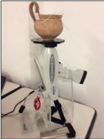
Figure 7. 1 An indigenous kyathos (FKY1) from Monte Finocchito positioned on the top of the Bruker III-SD for analysis.
