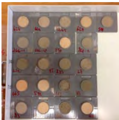
Figure 7. 17 Powdered samples in pressed pellets.
