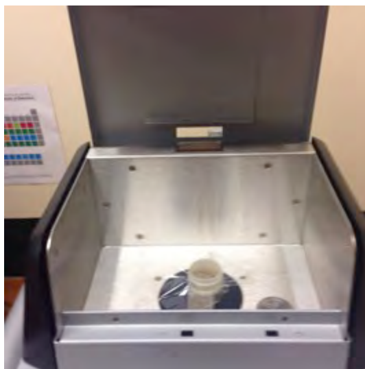
Figure 7. 18 Olympus DELTA Premium (DP 6000A): Pellet positioned on the Olympus test-stand.
