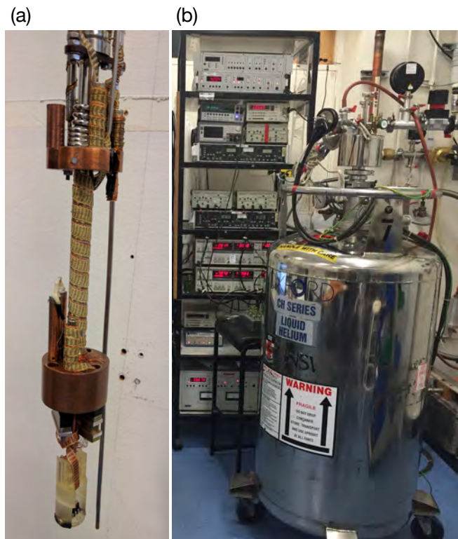
Figure 22: a) Picture of the end of the Heliox system, showing the 1K pot, and sample mount directly connected to the ^3\text{He} pot. (b) Picture of the Heliox fridge fully inserted into the liquid ^4\text{He} dewar next to the rack of measurement electronics.
