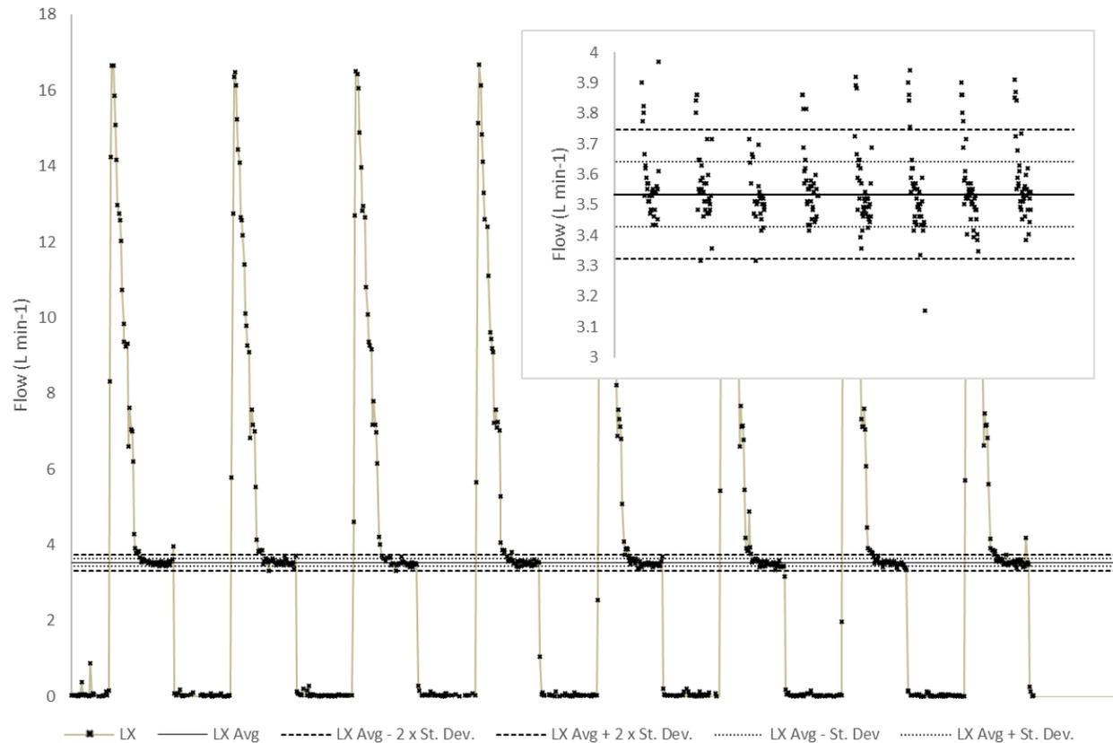
Figure 28 Sample of Left Exhaust Flow
