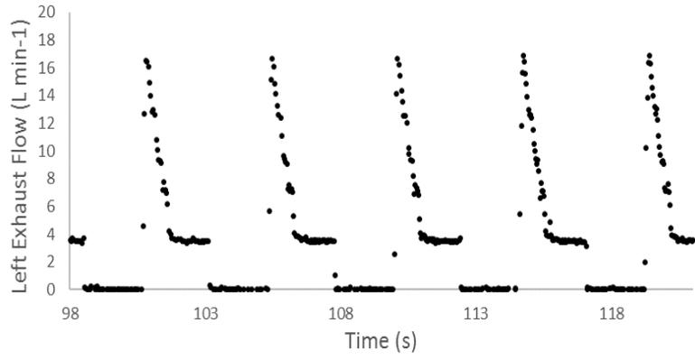
Figure 24 Sample left exhaust gas flow (breaths 3 - 7)
