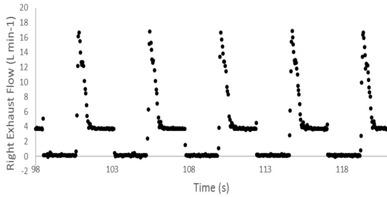
Figure 26 Sample right exhaust gas flow (breaths 3 - 7)
