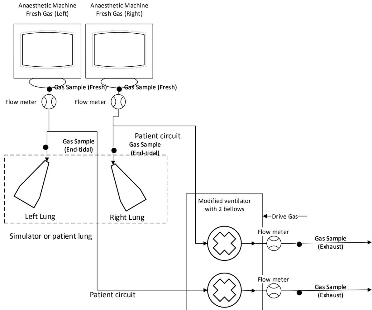
Figure 9 Measurement system for throughflow of isoflurane cardiac output
