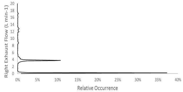
Figure 27 Right exhaust flow distribution
