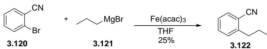
Figure 3.49: Kumada coupling of model Grignard reagent on 2-bromobenzonitrile to form 3.121 .
