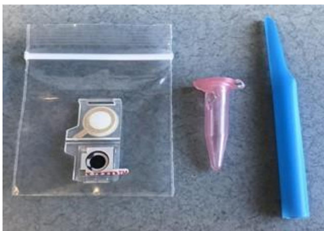
Figure 2-1. Researchers activated ION RAP cartridges manually. This included extracting gel from the pink tube using the blue straw and spreading it onto the black electrode surface of the cartridge
