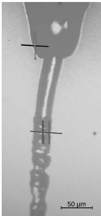
FIGURE 4.11: An image showing the HVI nozzle (top cross) with a stream of MyD88 crystals in LCP. The lower cross on the image indicates the location at which the sample and X-ray beam interact. The ripples of the sample (seen below the lower cross) demonstrate the effect of the X-ray beam on the sample after exposure.
