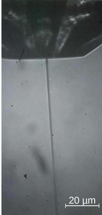
FIGURE 4.16: The tip of the GDVN nozzle (top) with the jet stream shown in this figure flowing from the nozzle vertically down.
