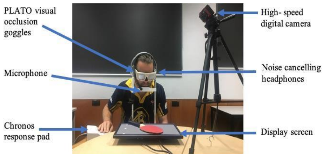
Figure 5.3. Experiment set up. Participants sat facing the screen with their head held stationary on a chin rest. Their right hand was placed on a button of a Chronos response pad. The visual occlusion goggles were coded to transition from transparent to occluded during the interstimulus interval (ISI) and inter-trial interval (ITI). The prime and target tools were either displayed on the LCD monitor or placed on top of the monitor. Participants wore noise cancelling headphones that played white noise throughout the experiment that masked external noise during stimulus changeovers. They also wore an interface microphone that recorded their verbal responses during catch trials.
