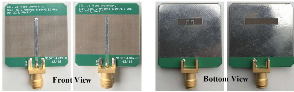
Figure 4-25. Photograph of the fabricated antennas. The proposed antenna is on the left side of each photo, whereas the conventional triangle slot antenna is on the right.
