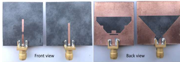
Figure 4-36. Photograph of the fabricated antennas. The proposed antenna is on the left side of each photo, whereas the simple triangle slot antenna is on the right.
