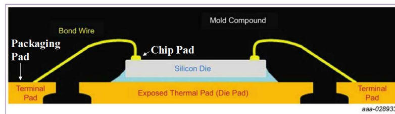
Figure 3-47. Bondwire in a chip [87].
