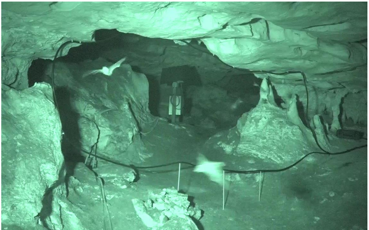
Figure 1. Southern bent-winged bats flying through the 15 m loop antenna which was installed at the restriction in Bat Cave. The bottom of the antenna-loop was raised above the cave-floor. Only a small area of the restriction (to the right of the
