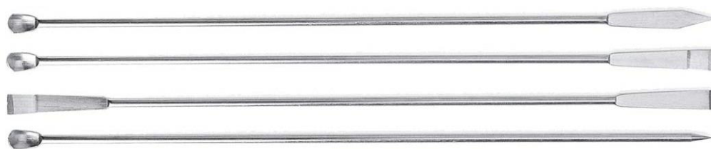
Figure 3. A collection of sharp metal micro-spatulas that were used to cut and extract frozen plasma samples.
