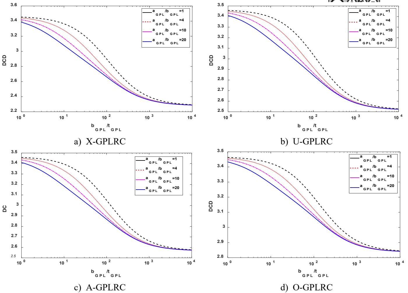
Figure 5: Effects of GPL geometry and dimension on the deflection of GPLRC C-C beams
