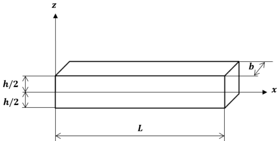
Figure 1. Geometry and co-ordinates of the studied beam
