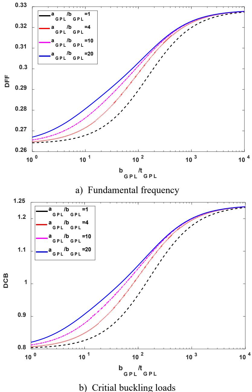
Figure 6: Effects of GPL geometry and dimension on the natural frequencies and critical buckling loads of X-GPLRC S-S beams ( $GG/h = 10$ ,  $WW_{GGGGG} = 0.1\%$ ,  $aa_{GGGGG} = 2.5 \times 10^{-6}$  )
