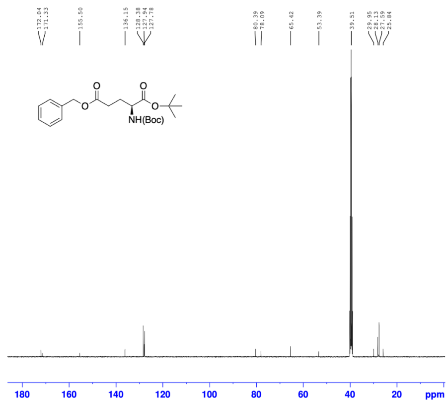
Figure 69 – Compound (17) ^{13}\text{C} -NMR obtained using 400 MHz Bruker NMR spectrometer in d_6 -DMSO
