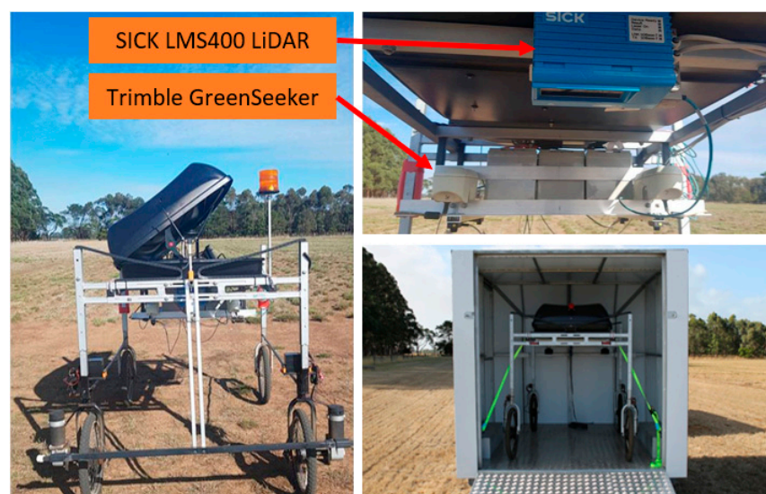
Figure 2. An unmanned ground vehicle (DairyBioBot) equipped with SICK LMS400 Light Detection and Ranging (LiDAR) unit and two Trimble GreenSeeker sensors operated at the Hamilton Centre experimental trial and was stored in the custom enclosed trailer. The trailer functions as a secure housing of the DairyBioBot as well as a base station for Real-Time Kinematic Global Positioning System (RTK GPS) navigation.
