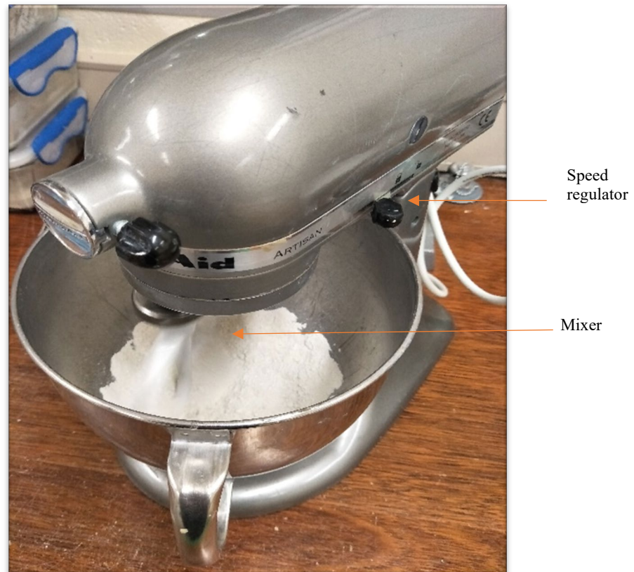
Figure 40: Automatic mortar mixer used in this study to mix dry soil samples at different moisture contents.
