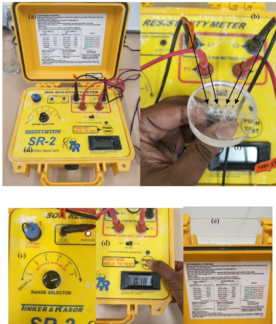
Figure 37: Soil resistivity meter and its specifications: a) complete set up, b) four pins representing four electrodes, c) range selector for resistance, d) a sample experiment, and e) information on the formulae for the conversion purpose.
