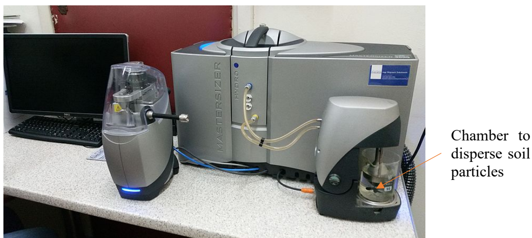
Figure 3.45: Malvern Mastersizer 3000 Laser Diffraction Particle Size Analyser setup.
