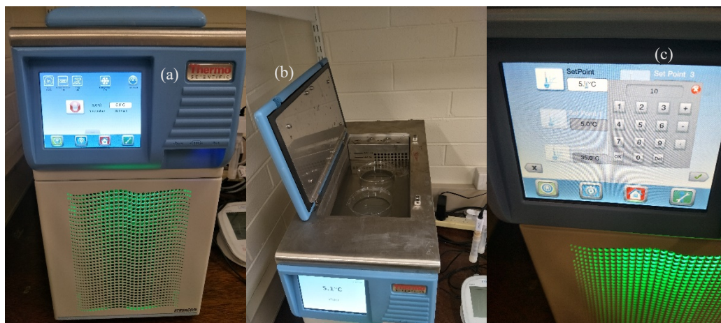
Figure 3.42: The optimised temperature controlling water bath used in this study: a) front set up of the device before starting the experiment, b) beakers are merged into the water to reach the targeted temperature, and c) display of keypad to enter the desired temperature input.
