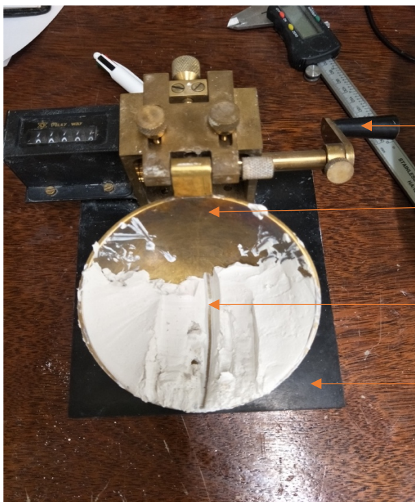
Figure 3.46: Sample Casagrande test to determine LL: a) groove creation before the actual test begins, and b) different parts of the Casagrande device.
