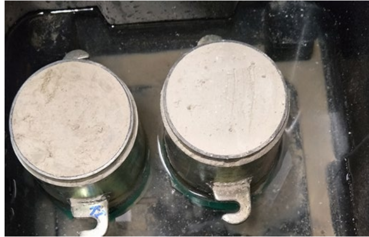
Figure 5.68: Saturation process inside a CBR soaking tank.
