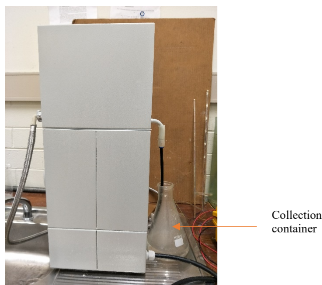
Figure 38: Heat-based distilled water maker.
