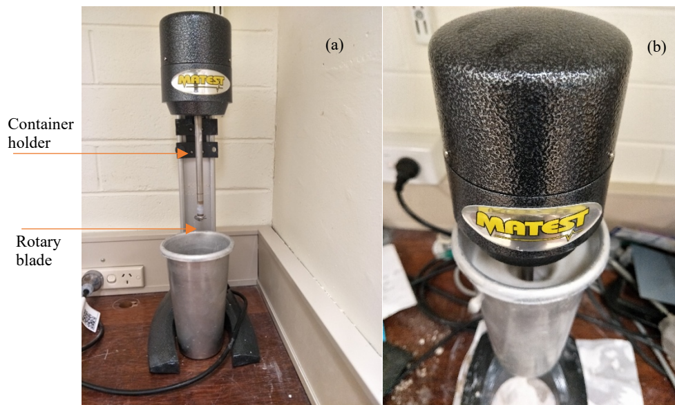
Figure 39: Soil-water suspension mixer used in this study: a) information on the parts of the device, and b) a sample mixing process ongoing.
