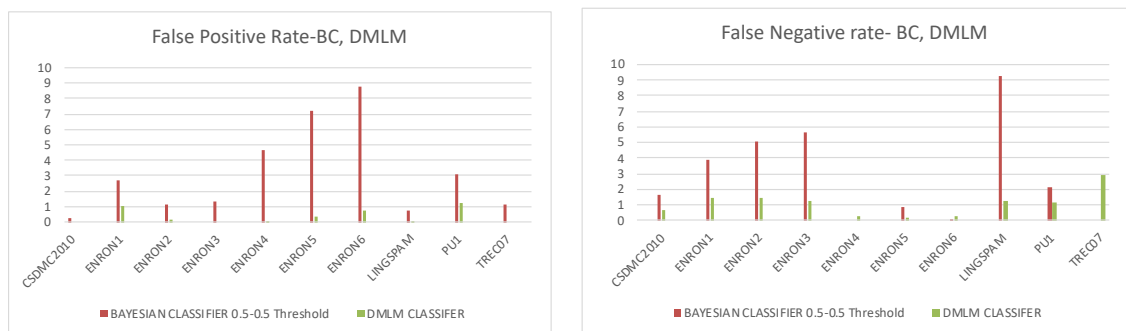
Figure 4.10: Graph showing a) False positive rate and b) False Negative for all 10 datasets for Bayesian classifier and DMLM
