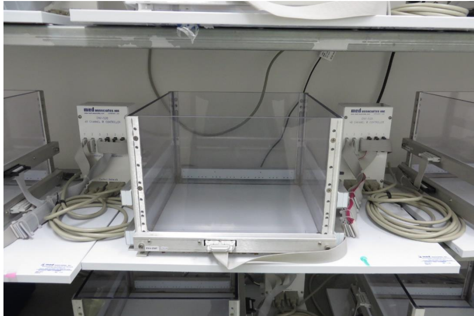
Figure 2.4 Mouse locomotor photocell arena. Mice are held in a clear box while locomotion is measured following acute injection. Photoelectric beam disruption records horizontal movement.
