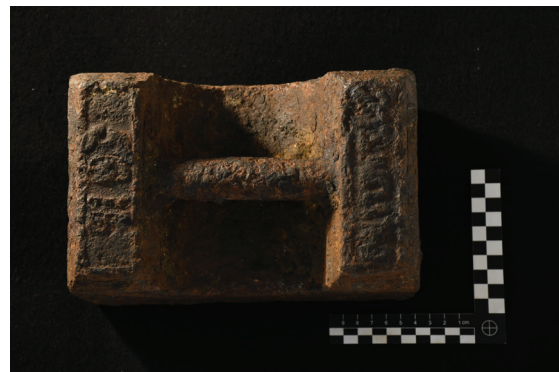
DW 08269 - calibrated bar weight
