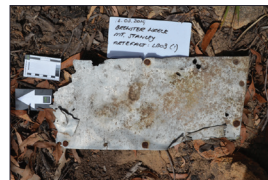
Left: Ammunition bay panel located at the Mount Stanley wreck site (photo by James Kightly, 2019) Right: The sole surviving Brewster Buffalo, with ammunition bays in wings circled (photo by Matt Sartenada via Dave Brown)
