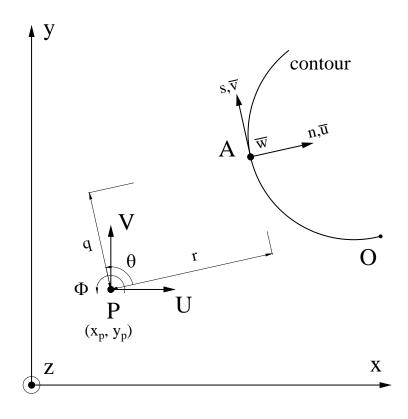
Figure 1: Coordinates for analysis of thin-walled beams.
