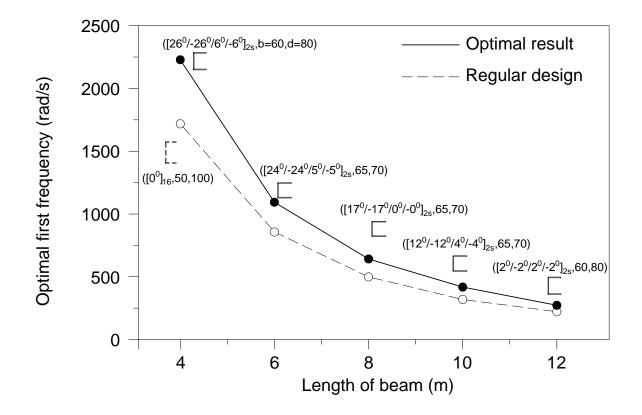
Figure 5: Vibration optimisation results for S-S beams with  $[\theta_1/-\theta_1/\theta_2/-\theta_2]_{2s}$  lay-up.
