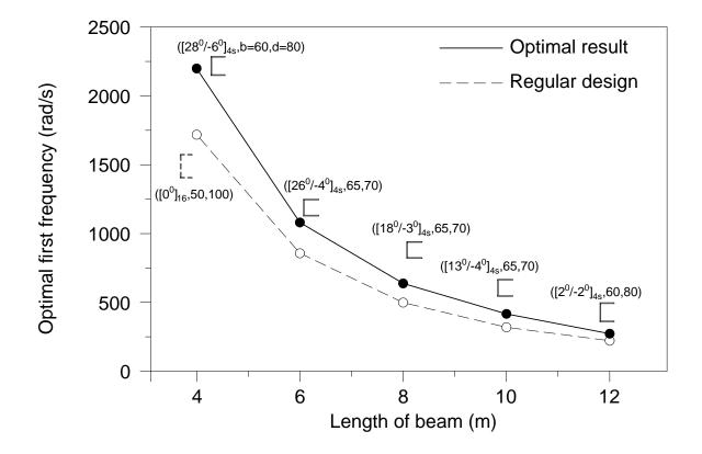
Figure 4: Vibration optimisation results for S-S beams with  $[\theta_1/-\theta_2]_{4s}$  lay-up.
