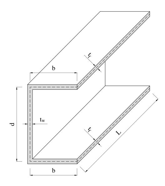
Figure 2: Geometry of a channel-section beam.
