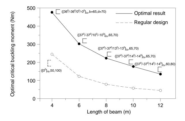
Figure 8: Lateral buckling optimisation results for S-S beams with  $[\theta_1/-\theta_1/\theta_2/-\theta_2]_{2s}$  lay-up.
