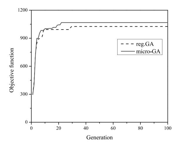
Figure 9: Convergence history of Vibration optimisation of a 6m-long S-S beam with  $[\theta_1/-\theta_1]_{4s}$  lay-up.
