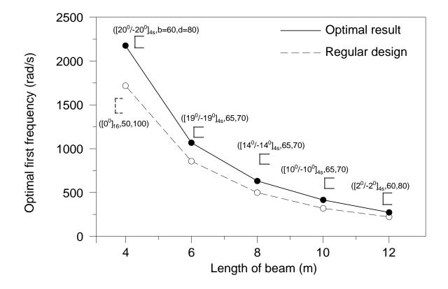
Figure 3: Vibration optimisation results for S-S beams with  $[\theta_1/-\theta_1]_{4s}$  lay-up.
