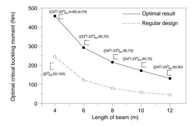
Figure 7: Lateral buckling optimisation results for S-S beams with  $[\theta_1/-\theta_2]_{4s}$  lay-up.
