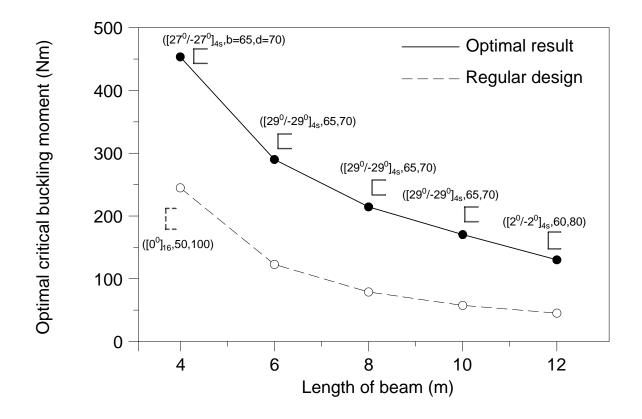
Figure 6: Lateral buckling optimisation results for S-S beams with  $[\theta_1/-\theta_1]_{4s}$  lay-up.
